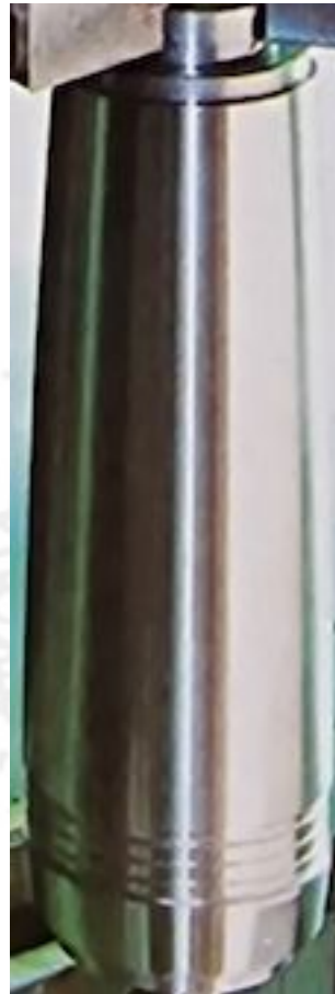
Forged 155 mm Howitzer Projectile Ready to Fill
